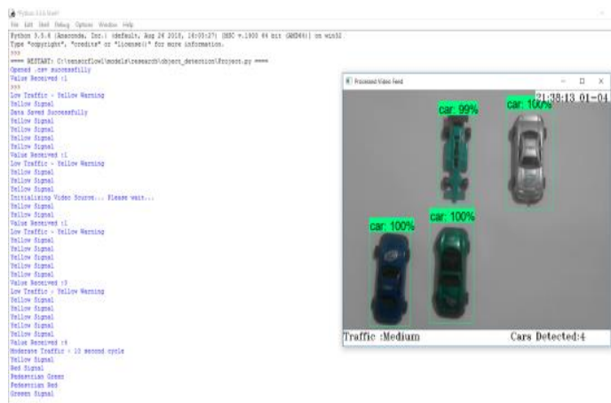
Fig. 3. Identification of Cars in Severe Traffic Situation
