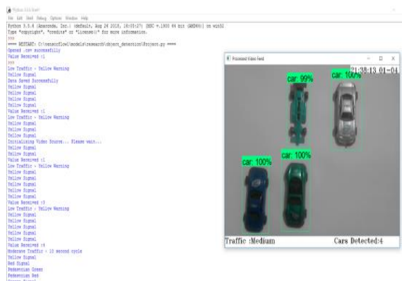
Fig. 2 Identification of Cars in medium density traffic
