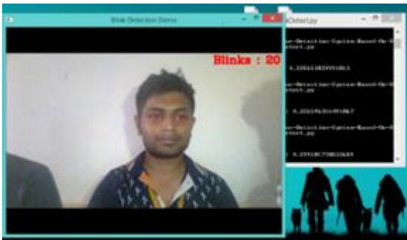
Figure 4. Reading the face and detecting eye regions and counting the blinks
