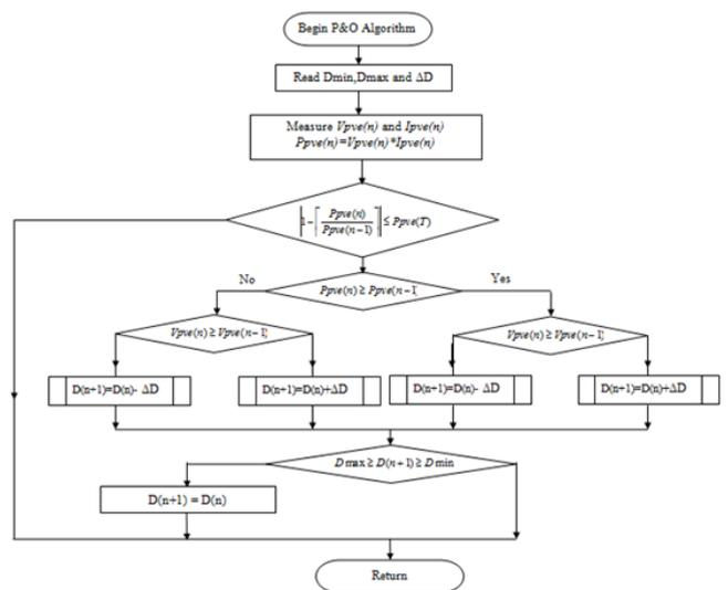
Figure 4.1 Proposed MPPT P&O algorithm flow chart
