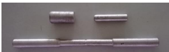
Fig 4 Photograph of the machined specimens (Hardness, Tensile test and Wear test)
