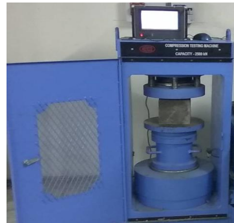
Figure 1: Compressive Strength test setup
