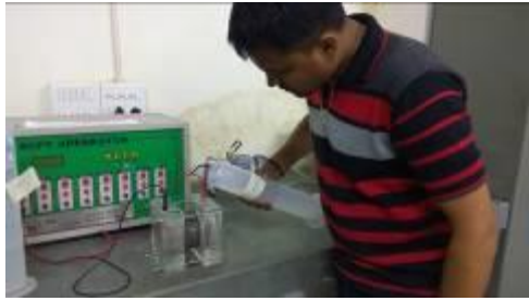
Figure 2: RCPT test setup
