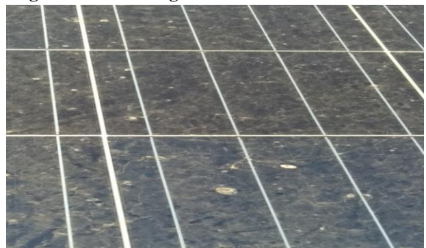
Figure 5 Shading due to Dirt-patches
