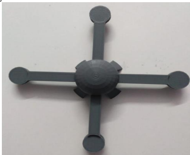
Fig. 10 3D printed optimized quadcopter frame
