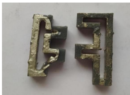
Fig.1: Fabricated IDE on glass substrate
