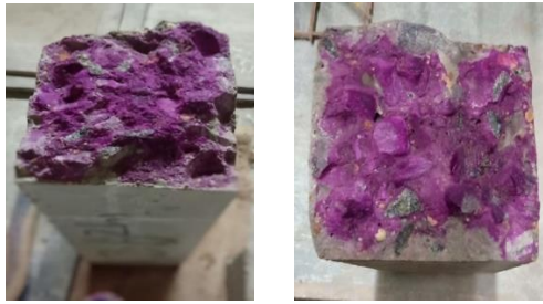
Fig: 12. Phenolphthalein test for water cured and CO 2 cured specimens
