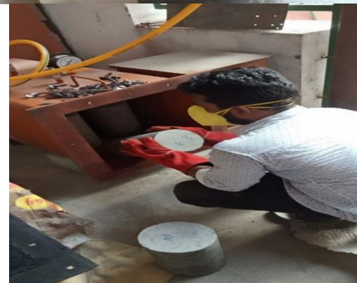
Fig: 2. Specimens in the CO 2 curing chamber
