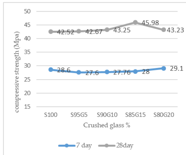
Fig 11: Compressive strength of concrete with Crushed glass
