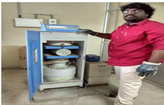
Fig 13: Split tensile specimen
