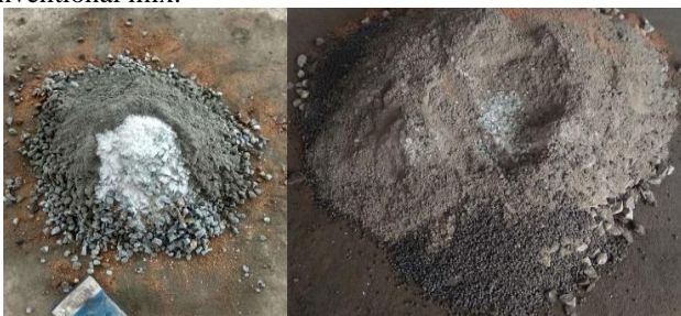
Fig 4: a) only crushed glass b) both crushed glass and plastic granules
