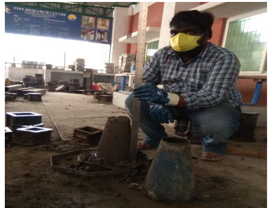
Fig 5: Measuring slump value
