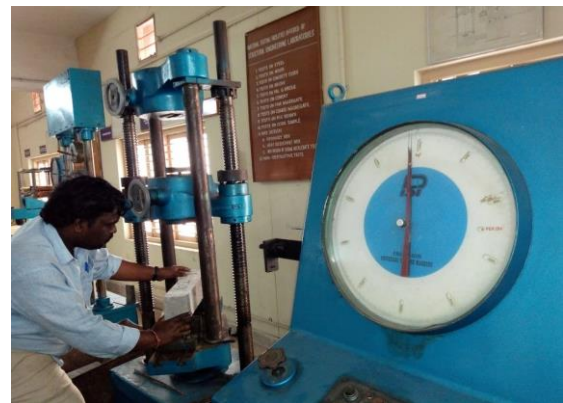
Fig 20: Flexural strength in Universal testing machine
