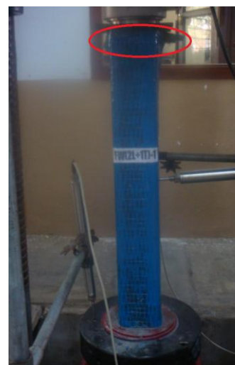
Fig. 12. Compression failure FW-[2L+1T]
