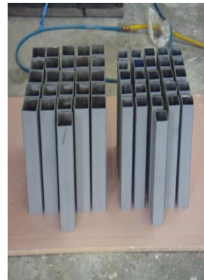
Fig.1. Columns after Sand Blasting
