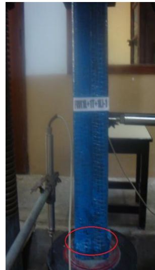
Fig. 11. Compression failure FW-[1L+1T+1L]
