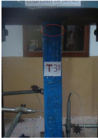
Fig. 7. Compression failure FW-[T3]
