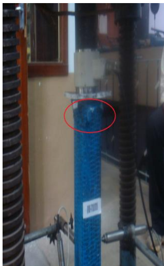
Fig. 9. Compression failure FW-[T1L1]
