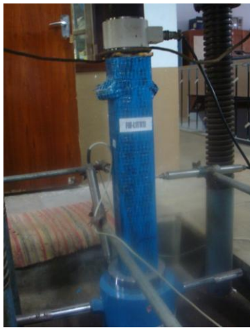
Fig. 8. Compression failure FW-[L1T1]
