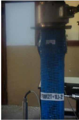
Fig.13. Compression failure FW-[2T+1L]
