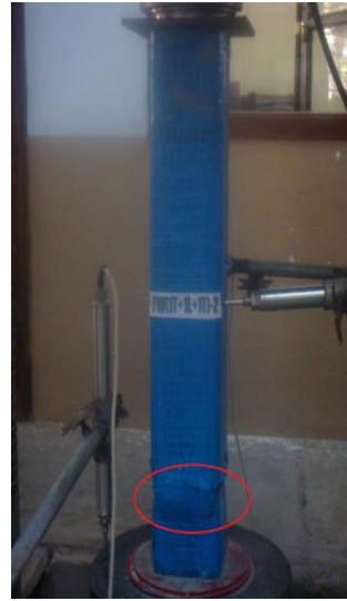
Fig. 10. Compression failure FW-[1T+1L+1T]
