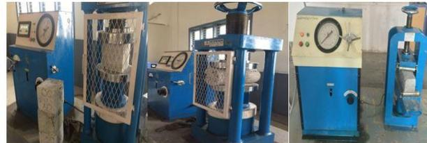
**Figure 2 Test setup for Compression, Tensile and Flexure Strengths**
