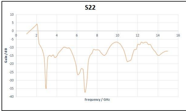
Fig 9. Measured S 22 using VNA
