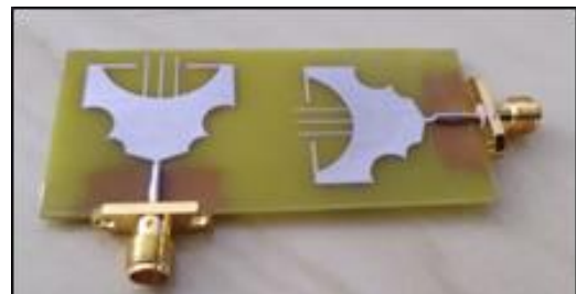
Fig 7. Top view of MIMO antenna prototype
