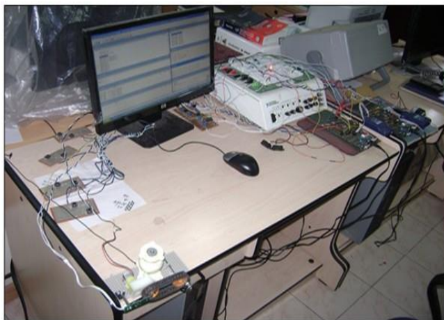
Fig.9. Experimental setup of elevator control system
