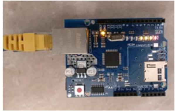
Figure 4: Ethernet Shield attached to Arduino at Parking Area
