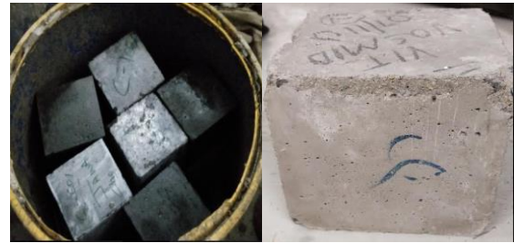
Figure 6: Tested specimens of chloride attack
