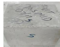
Figure 7: Tested specimens of sulphate attack
