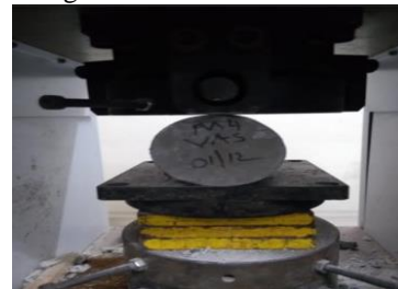
Figure 2: Experiment setup for split tensile test.
