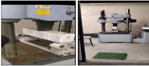
Figure 4: Experimental setup for flexural strength test
