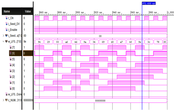
Fig.9: Simulated result of 8-bit LFSR
