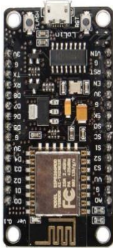
Fig. 5. Photo representing NodeMCU
