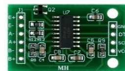
Fig. 4. Photo of load cell amplifier (HX711)
