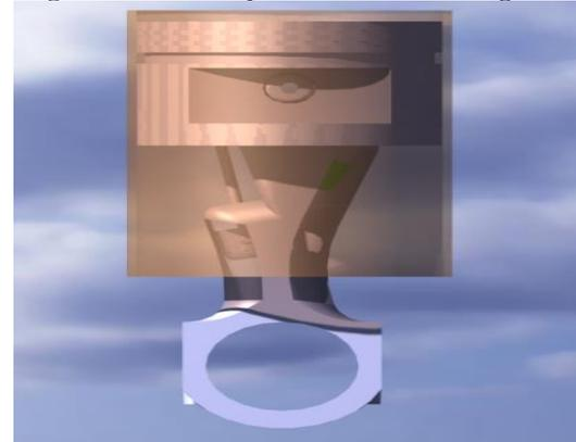
Fig.15 Front view of VCR Connecting Rod
