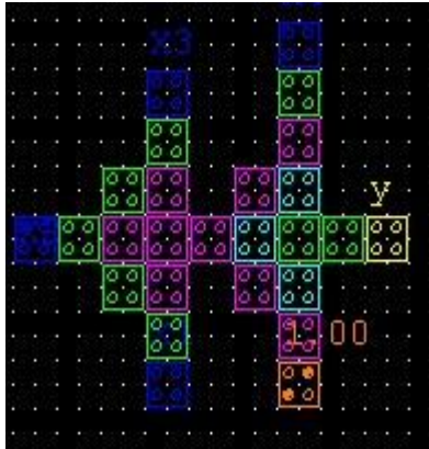
Fig. 6 4-bit odd parity generator
