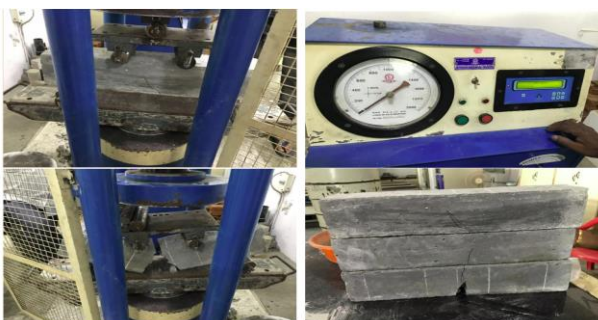
Fig One Point Load Testing on Beams
