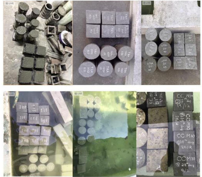
Fig 3 Casting and Curing of Specimens
