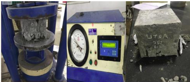
Fig 5 Compressive Strength Tests on cubes
