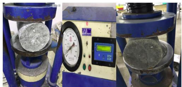
Fig 7 Split Tensile Strength Tests on cylinders
