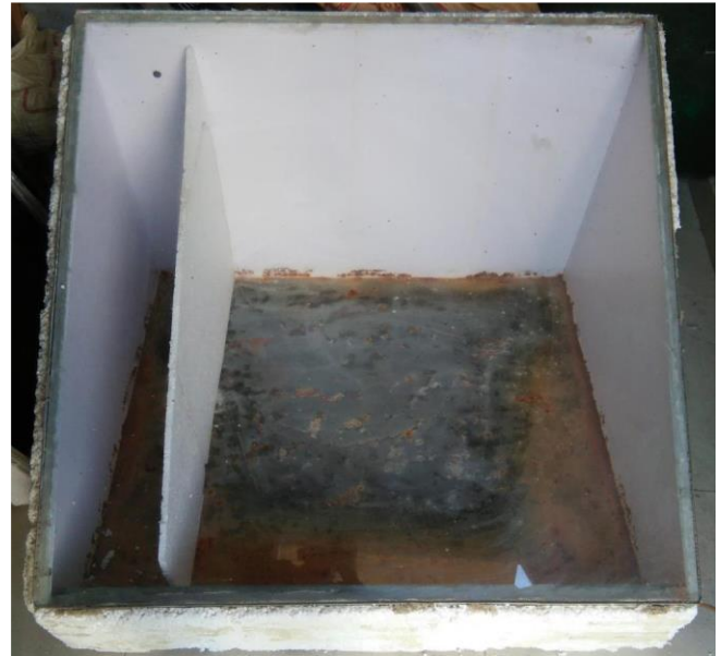
Figure 3 Experimental set up of solar still with separate condenser
