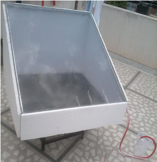
Experimental set up of simple solar still
