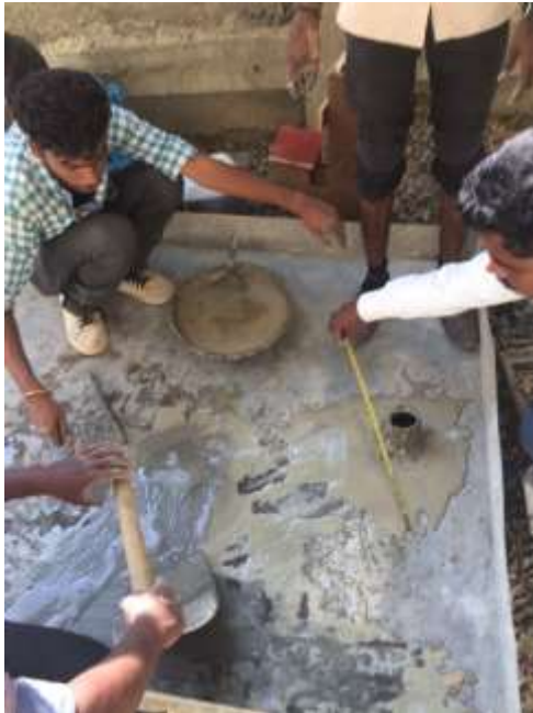
Photograph 1- Mixing and Minislump cone test
