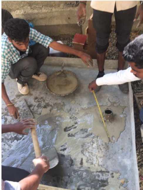
Photograph 1- Mixing and Minislump cone test
