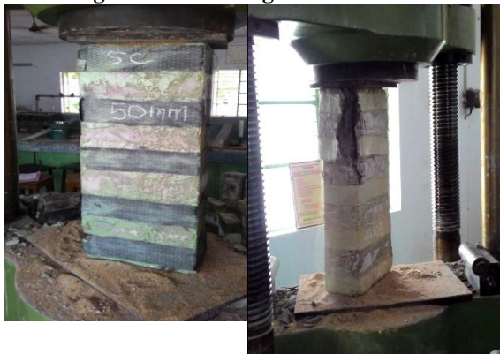
Fig 3:Testing of SC50 Fig 4:Failure of SG50
