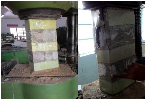
Fig 1 :Testing of SC83.33 Fig 2:Failure of SG83.33
