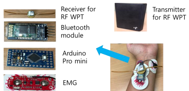
Figure 1. EMG sensor system using RF wireless power transmission method.
