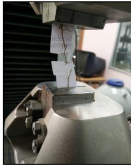
Figure 2: Root tensile strength test by Shimadzu Universal Testing machine
