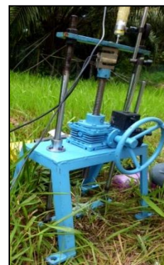
Figure 1: Fabrication of in situ pull out apparatus
