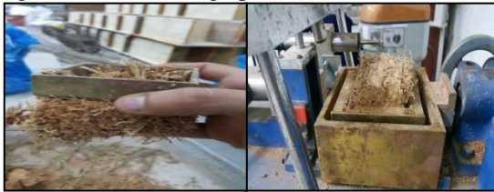
Figure 3: Soil with roots in the square box
