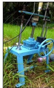
Figure 1: Fabrication of in situ pull out apparatus
