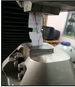
Figure 2: Root tensile strength test by Shimadzu Universal Testing machine
