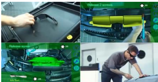
Fig.2: BMW augmented reality vehicle maintenance
