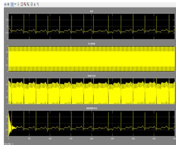
Figure 5. Output of Conventional 8-tap RLS filter using MatLab Simulink
