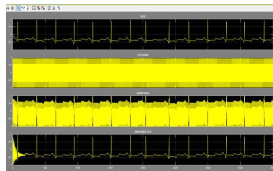
Figure 9. Output of Associativity 8-tap RLS filter using MatLab Simulink
