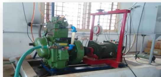
FIGURE 4.1: 4-Stroke, single cylinder diesel engine.
