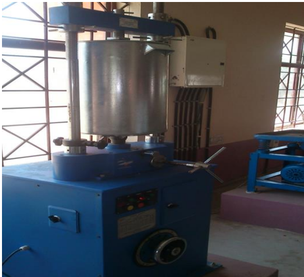
Fig.2 Test Setup – Load VS Settlement
