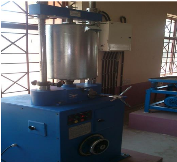
Fig.2 Test Setup – Load VS Settlement
