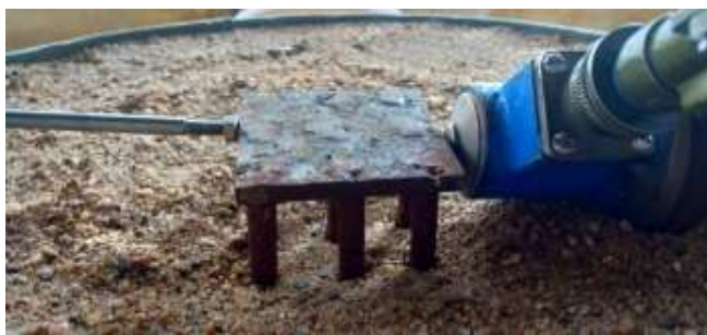
Fig. 4 Lateral loading setup
