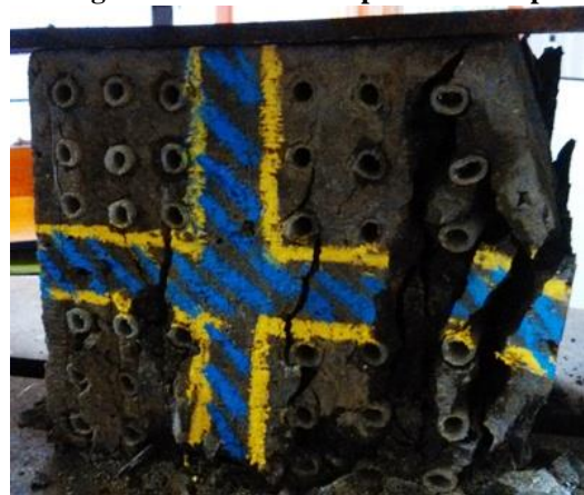
Fig.8 Cracking of cluster pattern test Specimen
