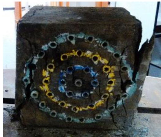
Fig.7 Cracking of concentric circle pattern test Specimen
