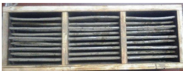
Fig.2 Test Specimen at Collapse
