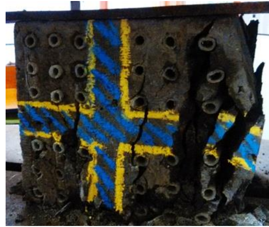
Fig.8 Cracking of cluster pattern test Specimen
