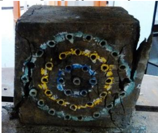
Fig.7 Cracking of concentric circle pattern test Specimen
