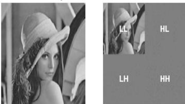
Figure 3: Base Image and its first level Decomposition
