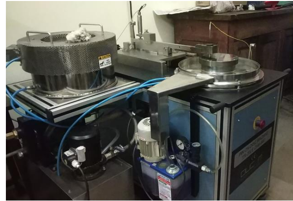
Figure -14 Ducom Rotary Tribometer with the heating chamber
