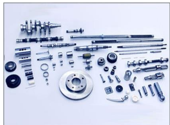
Fig1: Super finished Components.
