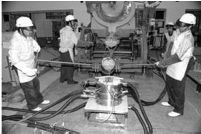
Figure 3. Melt transfer to ladle and pouring into EMS
