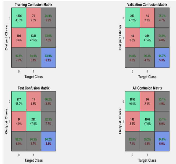
Fig. 16. All confusion matrix of fresh bearing and ball fault of 1000 micron
