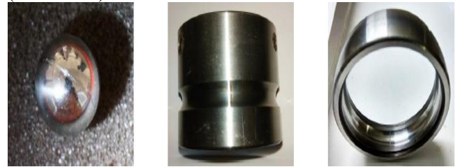
Fig. 3. Faulty bearing components (Ball, Inner race and Outer race)
