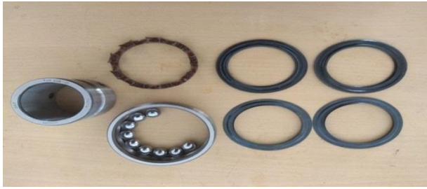
Fig. 2. Individual components of Deep groove ball bearing
