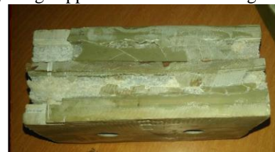
Figure No.1: Cracked Side View of Sample
