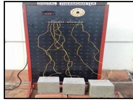
Fig. 3. Temperature Measurement Set-up (Digital Thermometer)
