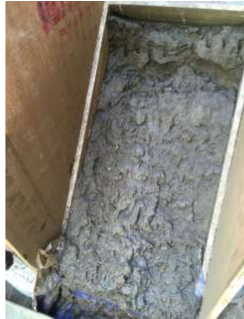
Fig 4: Soil erosion test with 40° slope
