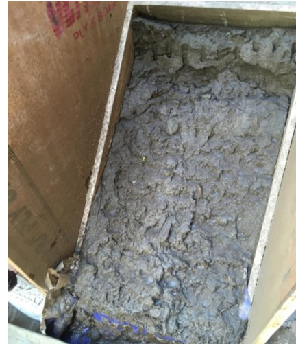
Fig 4: Soil erosion test with 40° slope
