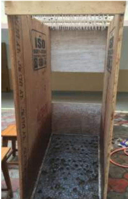
Fig 2: Soil erosion test with 20° inclination
