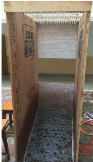
Fig 2: Soil erosion test with 20° inclination
