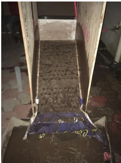
Fig 3: Soil erosion test with 30° inclination
