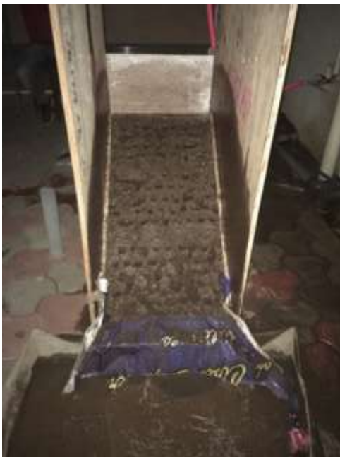
Fig 3: Soil erosion test with 30° inclination
