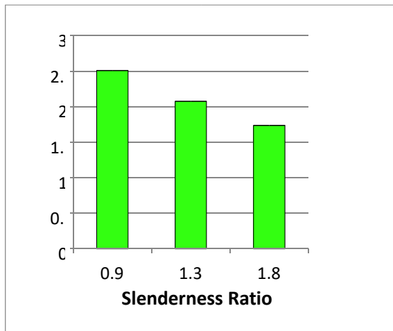
Fig.5. Strength Comparison of piers of different Slenderness Ratios made with Type 'B' bottles
