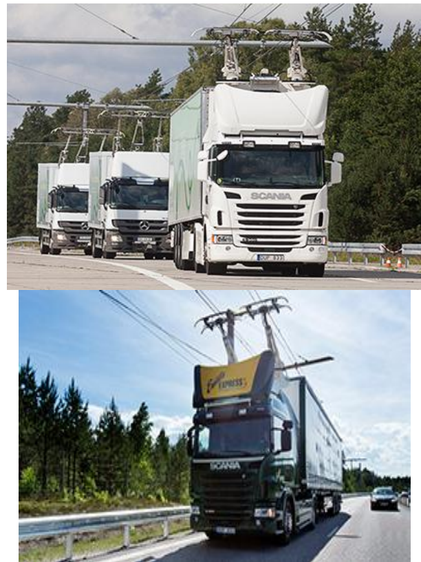
Figure 1. Illustrates a truck driving on an electrified road using overhead lines. (Source: Scania)
