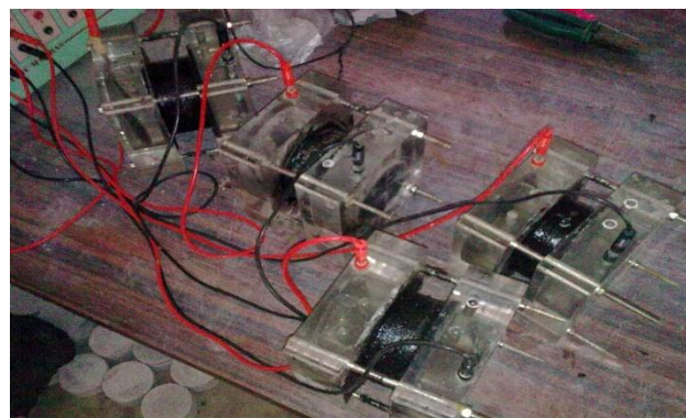
Figure:4 Experimental setup for RCPT test
