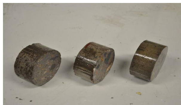
Figure:5 Cylindrical specimens for RCPT test
