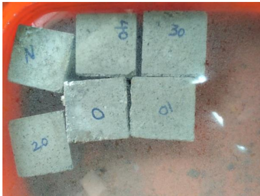
Figure 1 Specimens of SCC with HIPS granules in the water filled tank
