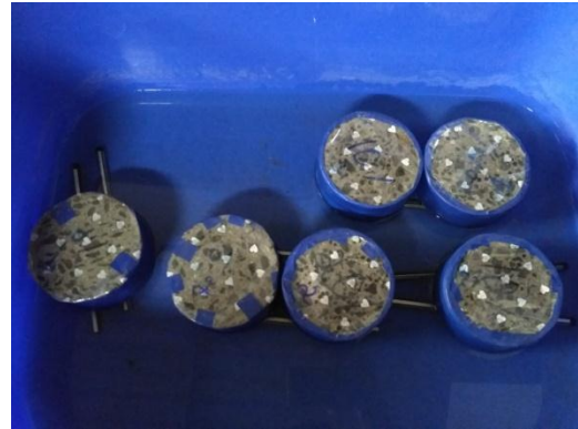
Figure 2 SCC specimens during Sorptivity test
