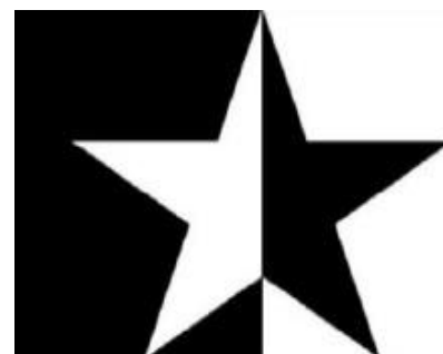
Fig (10) Self complementary structure
