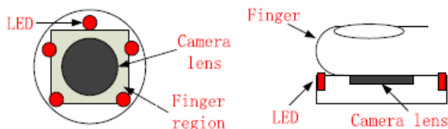
Fig 8. Acquisition of image in Non-Contact PPGi Method [28].
