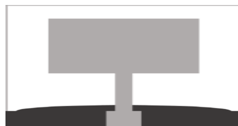
Fig (14) Planar monopole antenna
