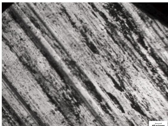
Figure 3.b. wear scar of uncoated substrate
