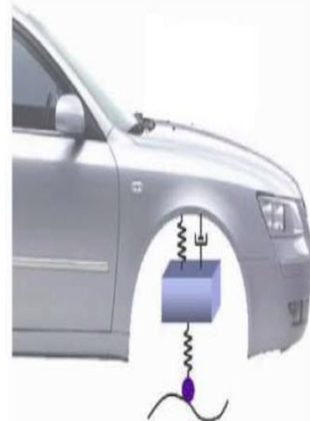
Fig.1. Schematic view of 1/4 car model
