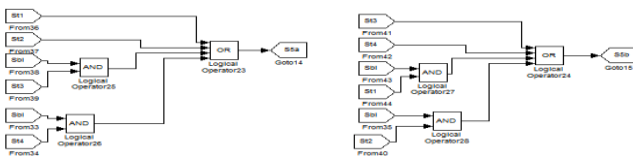
Figure 5 switching signal model of Matrix converter
