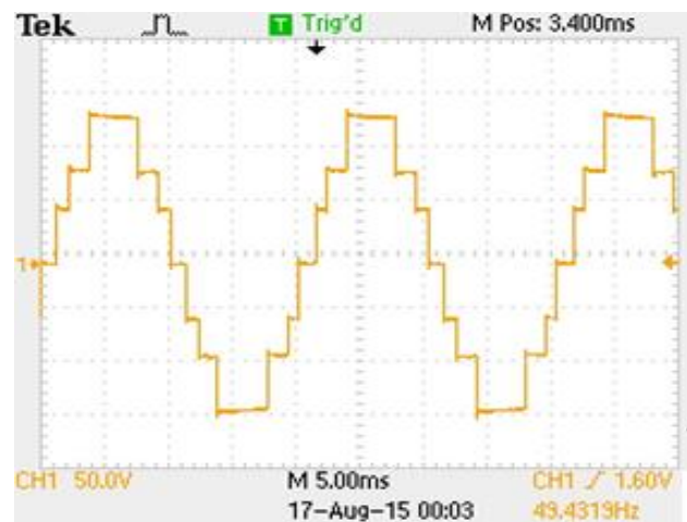
Fig.4. Output of seven level CHB MLI
